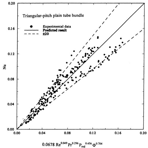
Fig. 11. Correlation of triangular-pitch plain tube bundle spray evaporation data.
