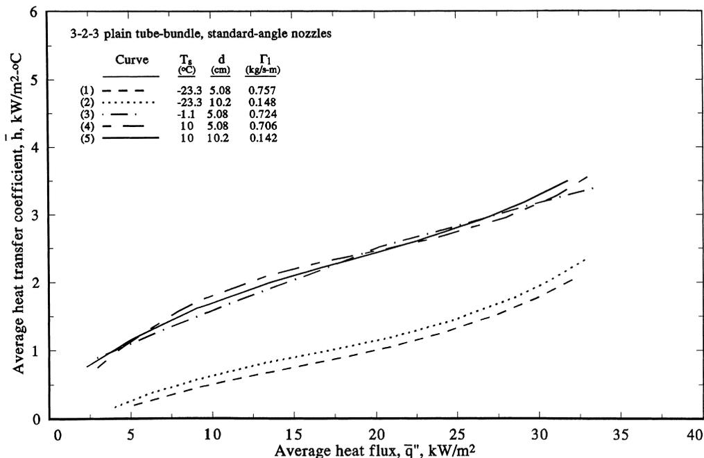
Fig. 1. Effect of saturation temperature on spray evaporation performance for standard-angle nozzles.
