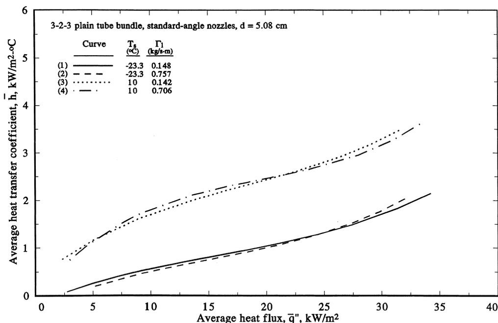
Fig. 6. Effect of spray flow rate on spray evaporation performance for standard-angle nozzles at  $d = 5.08$  cm.
