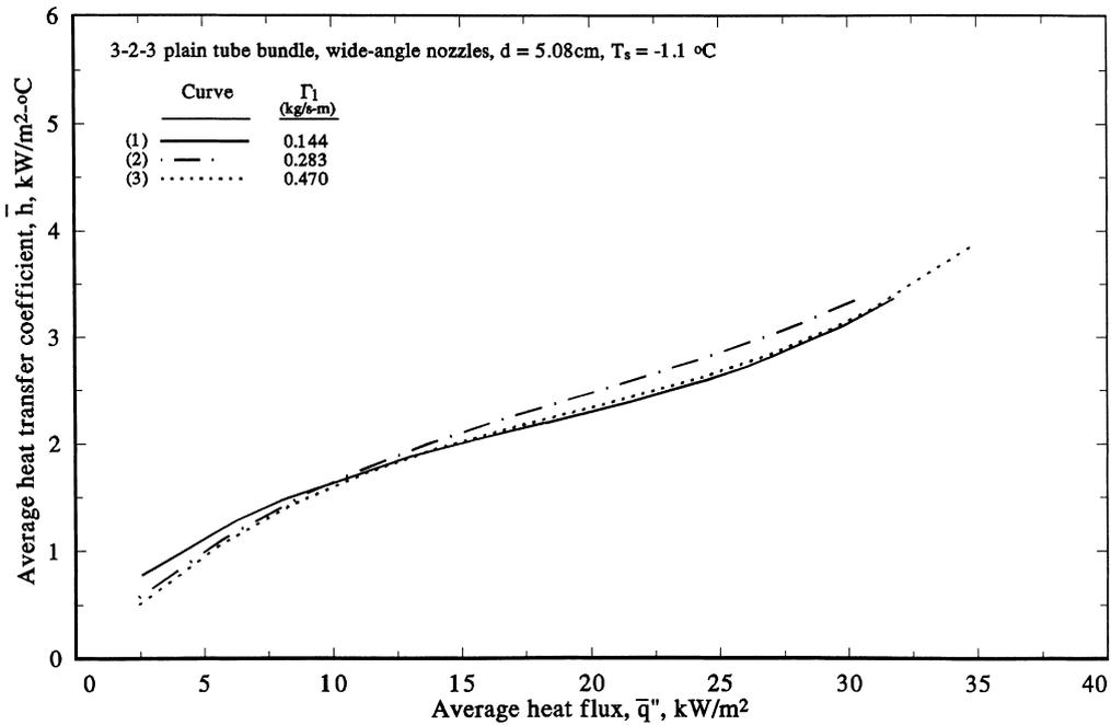
Fig. 5. Effect of spray flow rate on spray evaporation performance for wide-angle nozzles.
