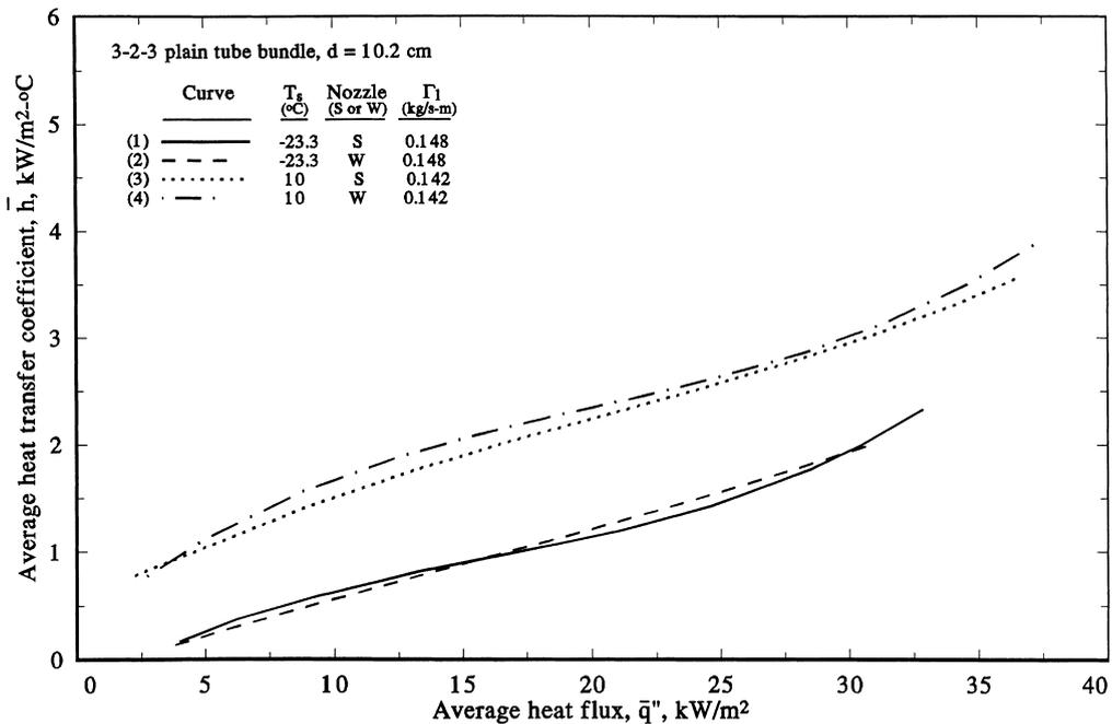
Fig. 10. Comparison of spray evaporation performance between standard-angle and wide-angle nozzles at  $d = 10.2$  cm.
