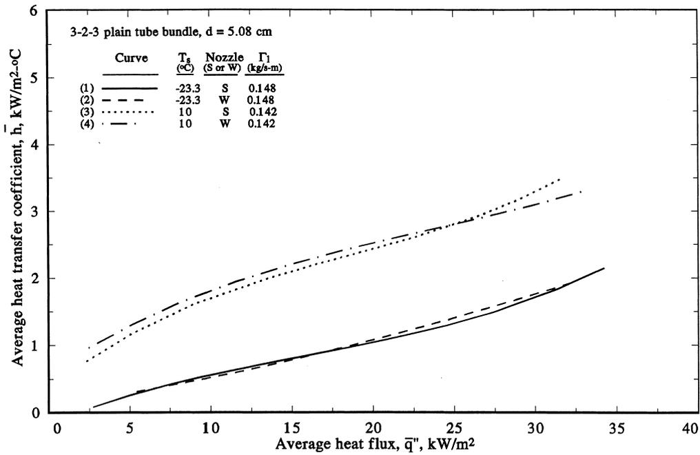
Fig. 9. Comparison of spray evaporation performance between standard-angle and wide-angle nozzles at  $d = 5.08$  cm.
