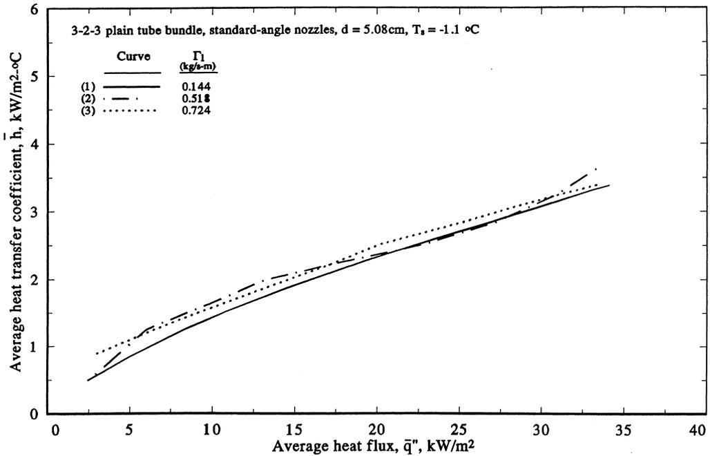
Fig. 4. Effect of spray flow rate on spray evaporation performance for standard-angle nozzles at  $-1.1\text{ }^\circ\text{C}$ .
