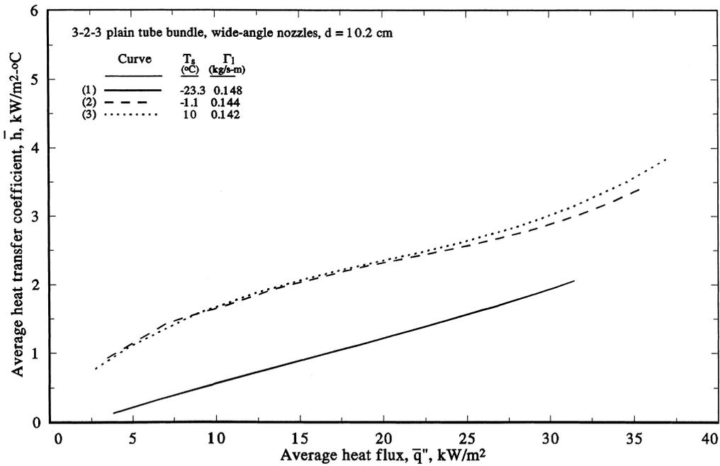
Fig. 2. Effect of saturation temperature on spray evaporation performance for wide-angle nozzles,  $d = 10.2$  cm.
