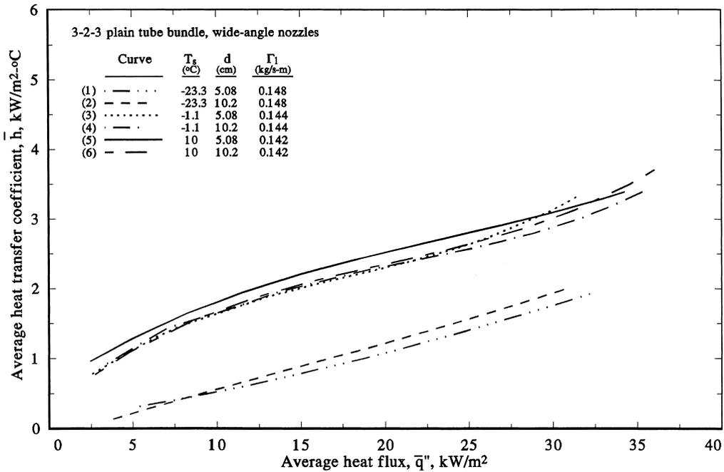
Fig. 8. Effect of nozzle height on spray evaporation performance for wide-angle nozzles.
