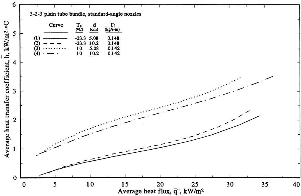
Fig. 7. Effect of nozzle height on spray evaporation performance for standard-angle nozzles.
