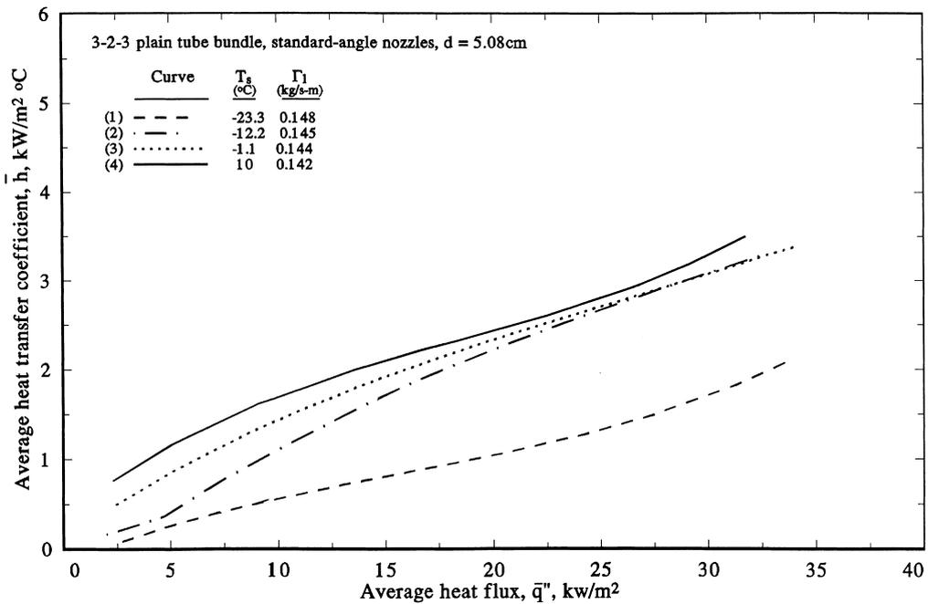
Fig. 3. Effect of saturation temperature on spray evaporation performance for standard-angle nozzles,  $d = 5.08$  cm.
